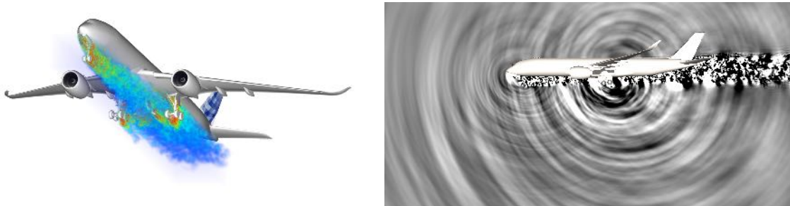
Figure 8: Illustration of LBM simulations in aerospace engineering. Left: take-off of A350 aircraft; Right: noise generated by landing gears on a full aircraft configuration during landing. Courtesy of Airbus. All simulations have been carried out with the ProLB software.
